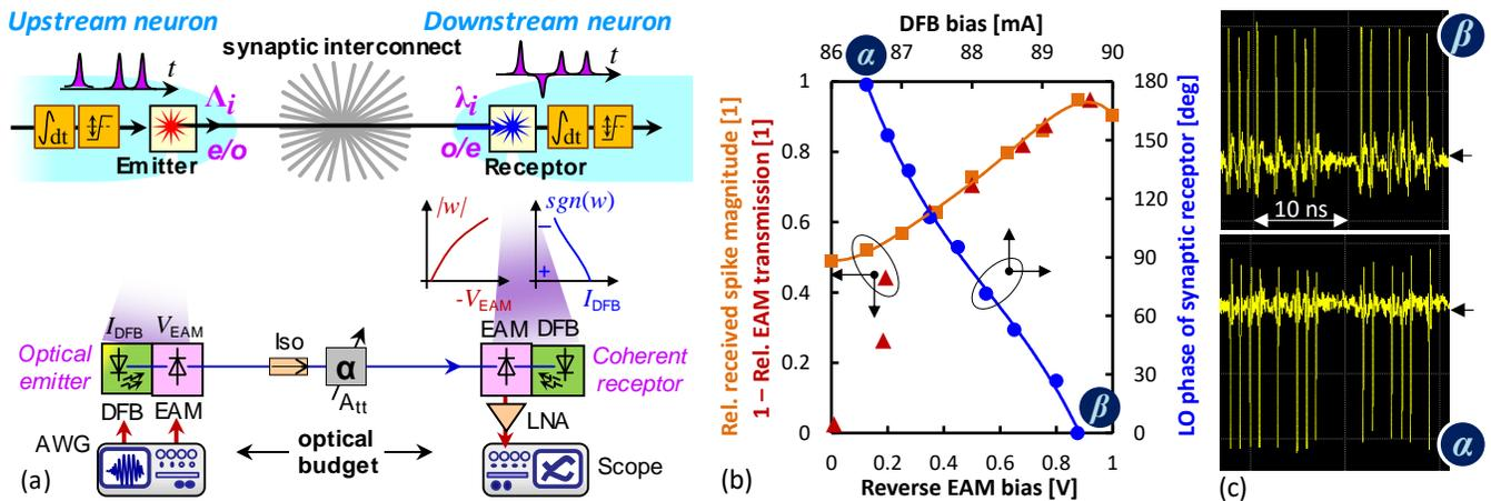
Fig. 2. (a) Concept and experimental setup for the coherent synaptic receptor. (b) Characterization of its integrated multiplication. (c) Received spike trains.
