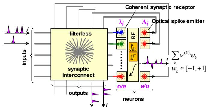
Fig. 1. Optical neural network with coherent synaptic receptors and filterless synaptic interconnect.
