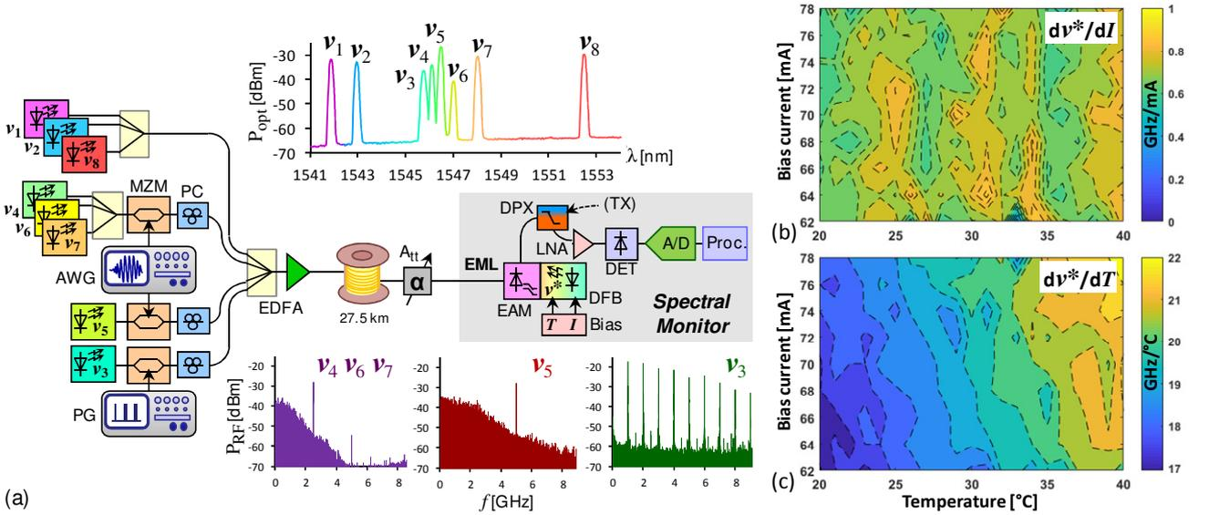
Fig. 2 (a) Experimental setup to evaluate the spectral monitor. The insets show the received optical spectrum and the electrical signal spectra at the particular channels. EML tuning efficiency for (b) current tuning and (c) temperature tuning.
