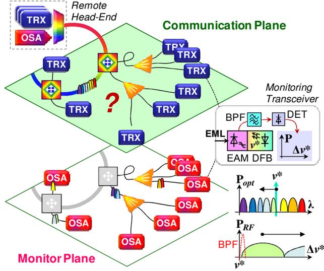
Fig. 1 Spectral monitoring integrated in EML transmitters.
